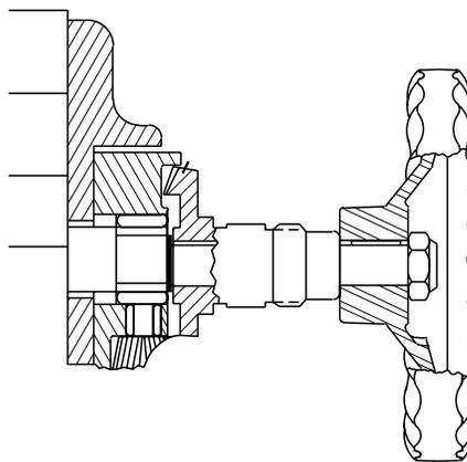
MANUALLY TURN HANDWHEEL. IF EXCESSIVE GEAR NOISE OR BINDING OCCURS, SHIMS NEED TO BE ADDED OR REMOVED, WHEN RE-SHIMMING, REPEAT STEPS 1 AND 2.
