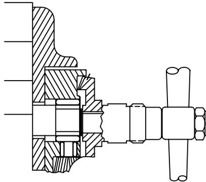
WITH POWER FEED IN NEUTRAL POSITION, TURN HANDCRANK. IF EXCESSIVE GEAR NOISE OR BINDING OCCURS, SHIMS NEED TO BE ADDED. WHEN ADDING SHIMS, REPEAT STEPS 1 AND 2.
