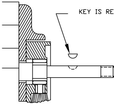
KEY IS REMOVED DURING SHIMMING
